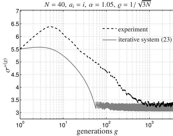
Figure 7: Illustration of the effect of  $\hat{\Delta}$  cumulation (26) on the normalized mutation strength dynamics of the  $[1, 2(3/3_I, 10)^1]$ -Meta-ES. Again, the solid line represent the predictions of the iterative system (23). The experimental results are averaged over  $10^3$  independent Meta-ES runs and illustrated by the dashed line.
