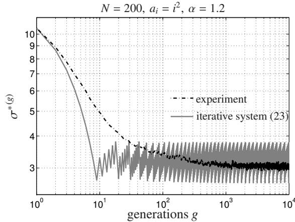
Figure 4: The normalized mutation strength dynamics of the  $[1, 2(3/3_l, 10)^1]$ -Meta-ES plotted against the number of generations. The predictions resulting from iterative system (23) are compared to real Meta-ES runs. The experimental results are averaged over  $10^3$  independent runs.
