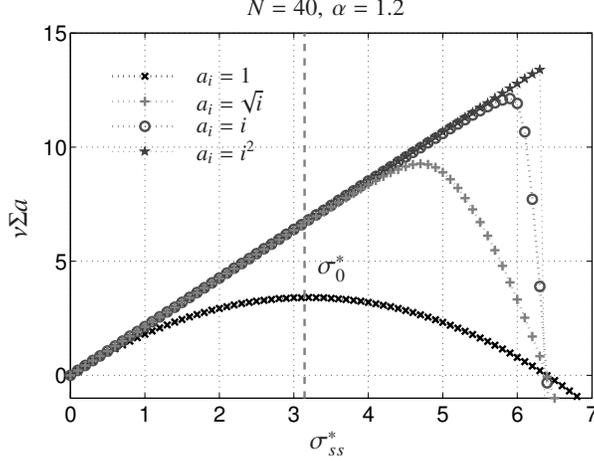
Figure 13: Numerical solutions of the eigenvalue problem (51) plotted against the normalized steady state mutation strength  $\sigma_{ss}^*$ . The results of four different ellipsoid models,  $a_i = 1$ ,  $a_i = \sqrt{i}$ ,  $a_i = i$ , and  $a_i = i^2$ , are displayed using the  $[1, 2(3/3\gamma, 10)^1]$ -Meta-ES with  $\alpha = 1.2$  in search space dimension  $N = 40$ . The point of discontinuity (39) is illustrated by the vertical dashed line.
