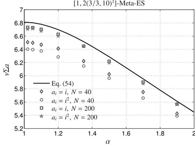
Figure 14: Product of the eigenvalues (54) and the sum of the ellipsoid coefficients  $\Sigma a$  plotted against the interval of control parameters  $\alpha$ . The experimentally obtained values on the ellipsoid models  $a_i = i$ , and  $a_i = i^2$ , are displayed as data points in search space dimensions  $N = 40$  and  $N = 200$ .
