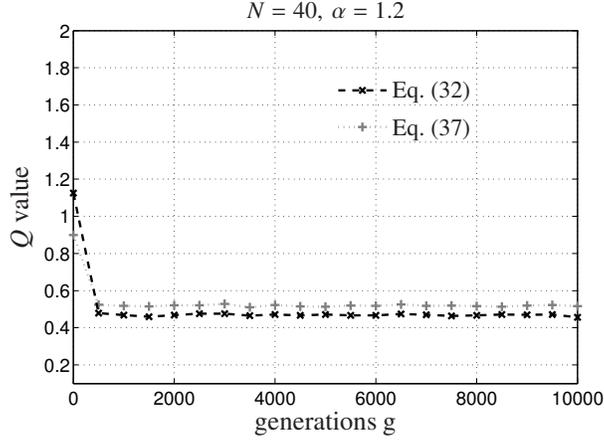
Figure 8: The  $Q$  value dynamics of the  $[1, 2(3/3_I, 10)^1]$ -Meta-ES on the ellipsoid model ( $a_i = i$ ). The strategy is initialized at  $y_i^{(0)} = 1 \forall i$  with  $\sigma_0 = 1$ .
